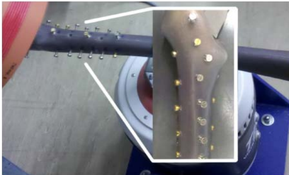
Fig. 14. Measurement setup focusing on a variation of the loosening state. Hereby prosthesis is integrated in an artificial bone. An adjustable anchorage is reached by fastening or loosening off screws evenly distributed around the prosthesis.
